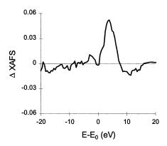
Fig. 4.  $\Delta L_{II} = L_{II}(H_2 – Pt) - L_{II}(Pt) = \Delta XAFS$  for Pt/LTL (1.25).
