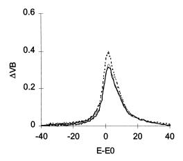
Fig. 5.  $L_{III}(Pt) - L_{II}(Pt) = \Delta VB$ ; (thin solid) Pt/LTL (0.63); (dotted) Pt/LTL (0.96); (bold solid) Pt/LTL (1.25).
